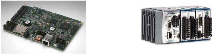
Fig. 2. Single board RIO (LHS) targeted for OEM applications and the more powerful cRIO (RHS).
